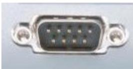
If you are connecting to a standard Serial port (pictured left) then it is most likely Com Port 1 or 2 and may be labeled on the PC.
